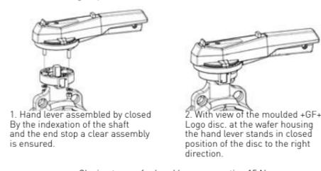
Closing torque for hand lever connection 15 Nm
